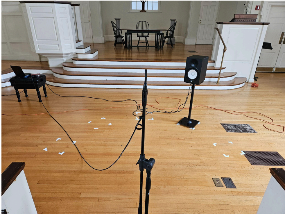
Figure 5.1.5: Position of Speakers and Microphone from Microphone View for PCCH
