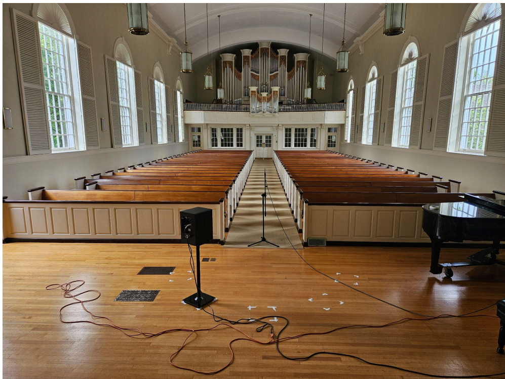
Figure 5.1.6: Position of Speakers and Microphone from Speaker View for PCCH
