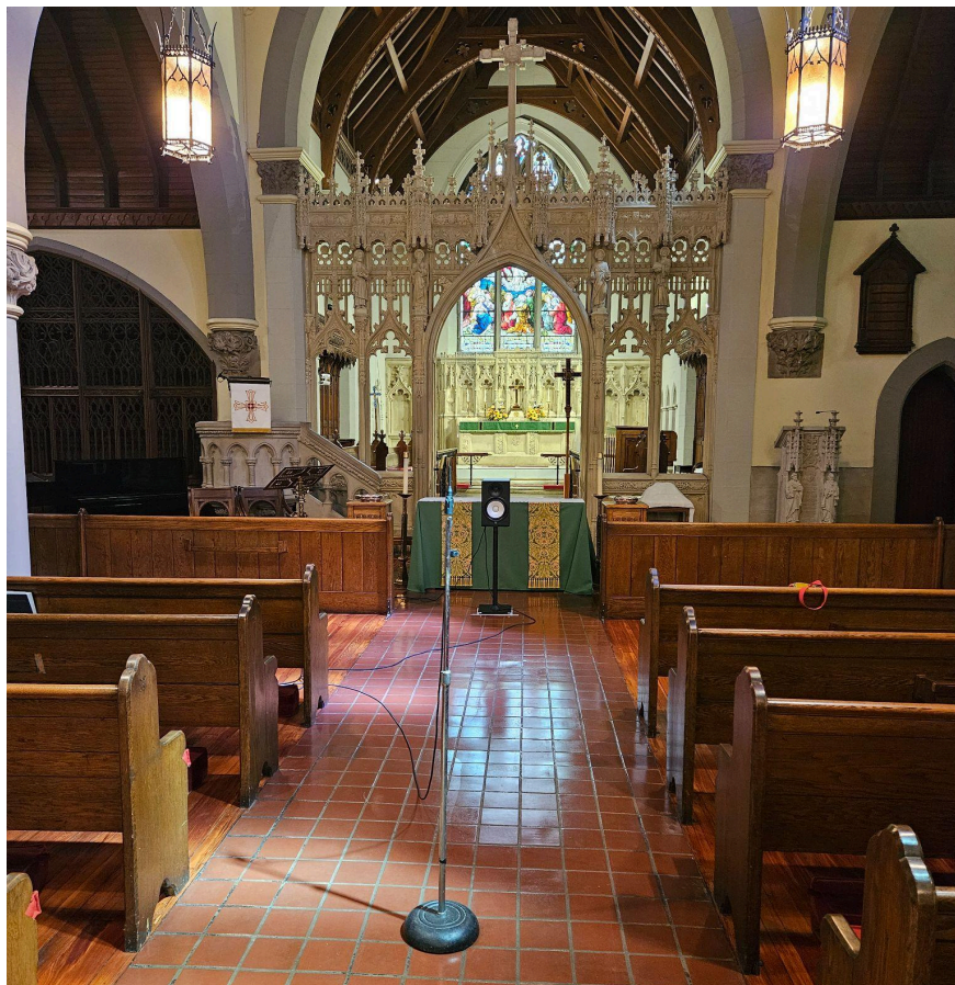
Figure 5.1.19: Measurement Microphone Placement for GEEC
